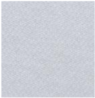
INTERLOCK KNIT A double-knit fabric with a smooth surface on both sides, offering a soft hand feel and good stretch, commonly used in t-shirts and underwear.
