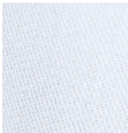
TWILL WEAVE A fabric characterized by a discreet diagonal rib pattern, offering durability and a soft drape, commonly used in shirts and trousers.
