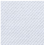
OXFORD WEAVE A basket weave fabric combining two yarns woven together, resulting in a slightly textured, soft, and breathable finish, ideal for both casual and formal shirts.
